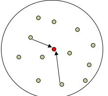
Nodes communicate with the sink via possibly multi-hop routes by using peer nodes as relays. With fixed transmission range, nodes closer to the sink will serve as relay for a larger number of sources. We assume that all sources use the same frequency to transmit data, thus sharing time. However, the results apply as long as there is a single shared resource, e.g., time, frequency, and so on.
